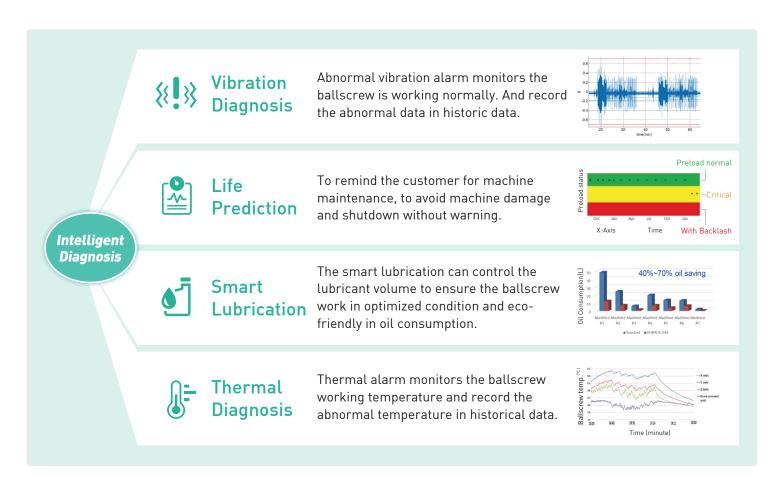
i4.0BS<sub>®</sub> transmits signals via sensors and PLC I/O to the edge computing module for calculation and analysis. Then the results are shown on display devices through Ethernet network to achieve remote monitoring.
