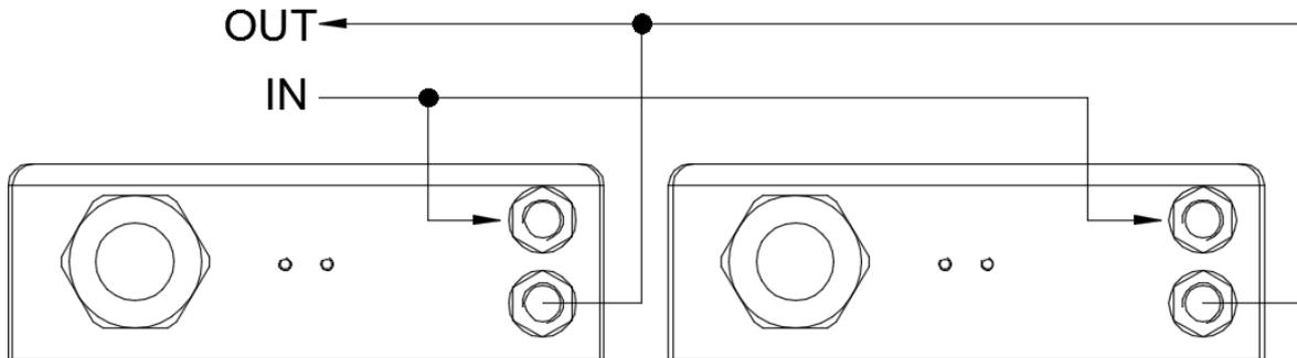
Fig.16 The diagram of motor cooling circuit installation
