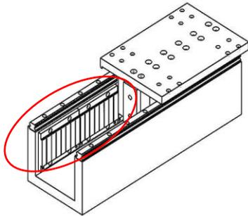
2. Place the non-magnetic material in between the interface of the stators on two sides.
