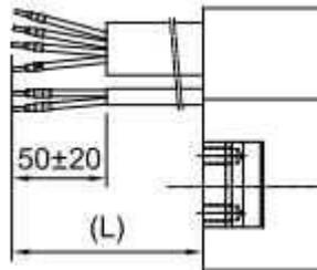
Fig. 18 Outlet Specifications for a Power Cable
