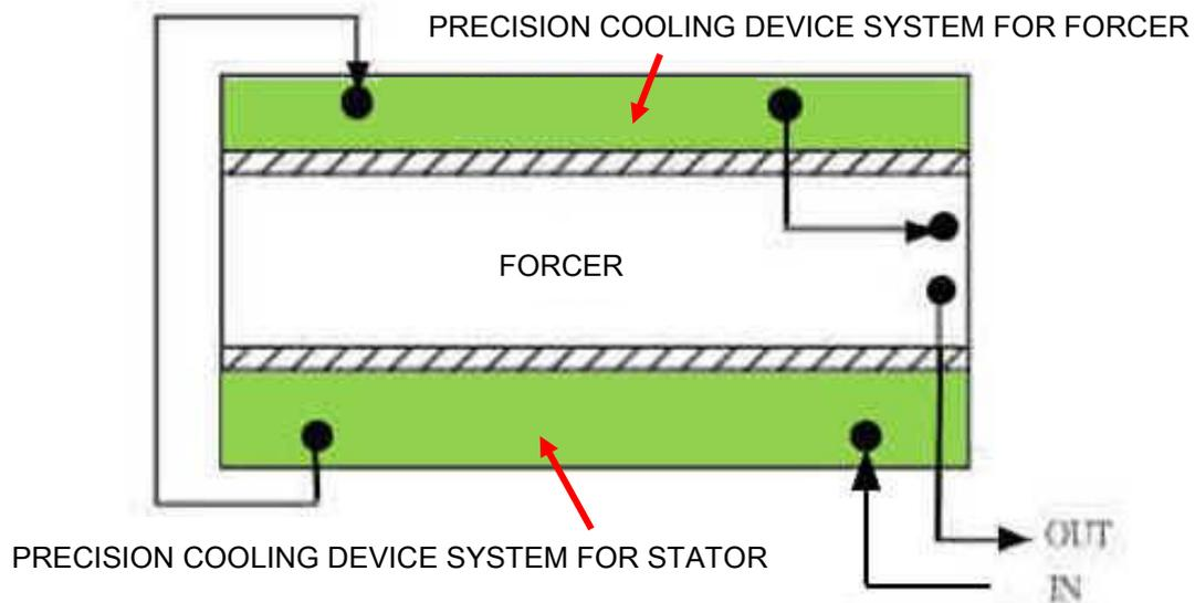
Fig. 17 The diagram of runner of precision cooling device
