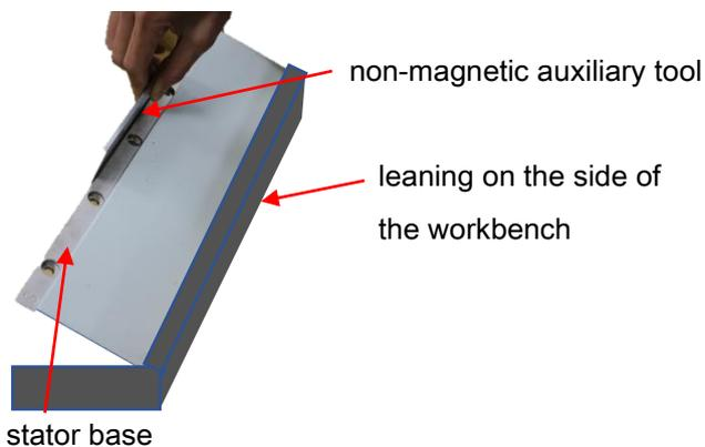
Fig. 8 Stator leans on one side with the non-magnetic auxiliary tool, handling the stator by its base.
