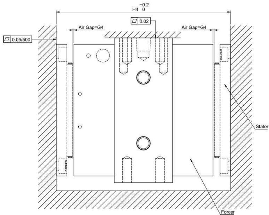
Fig.5 LMSC double thrust linear motor assembly
