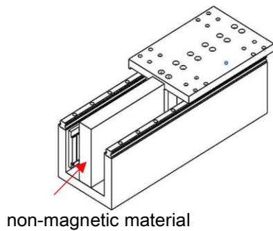
3. Use a non-magnetic tool to install the stators on the other side of half of the stroke.
