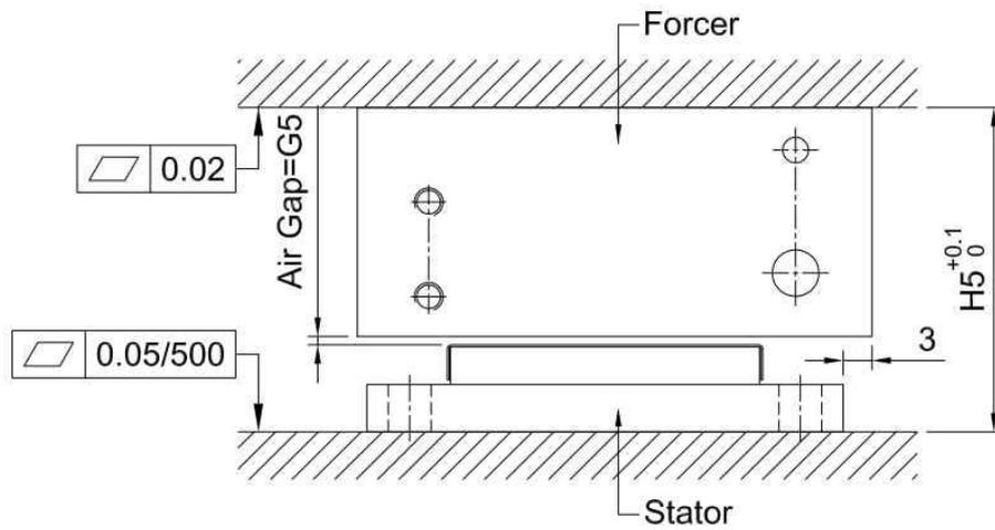
Fig.6 LMSS linear motor assembly
