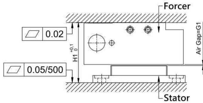
Fig. 2 LMSA linear motor assembly
