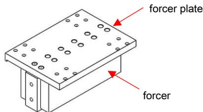
2. Install the forcer plate on the block.
