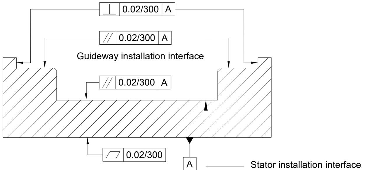
Fig. 1 The sectional view of base design
