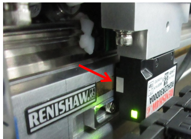
(b) Renishaw encoder gap is 0.8 \pm 0.15 mm
