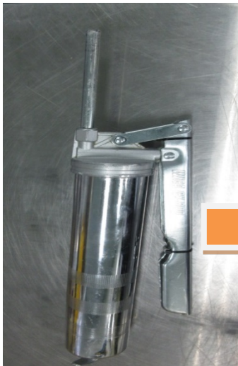
(a) Fill-in the grease
