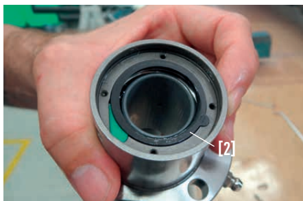
Fig. 4.13 NBR wiper [2] and support ring [1]
