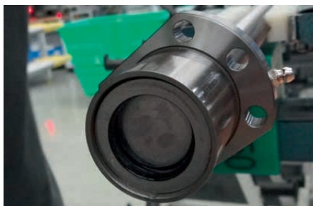
Fig. 4.10 Removing the metal ring
