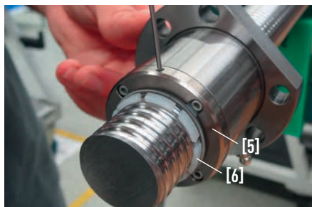
Fig. 4.14 Loosening the grub screws
