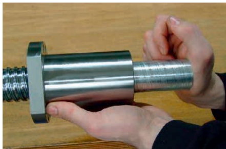
Fig. 4.6 Screw nut with wiper onto shaft
