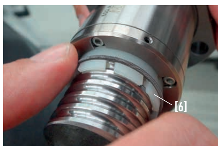
Fig. 4.15 Removing the finger wiper
