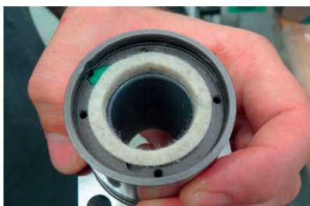
Fig. 4.12 Nut with inserted felt wiper
