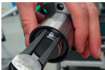
Fig. 4.9 Removing the circlip
