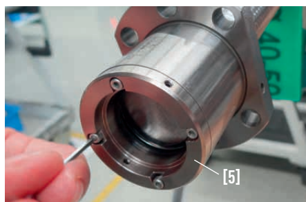
Fig. 4.16 Unscrewing the wiper housing
