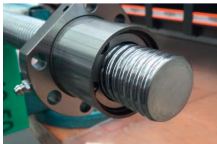
Fig. 4.8 Nut at the end of the shaft
