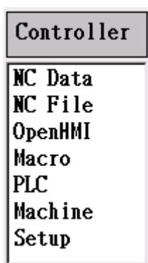
Display the file type that current login permissions can access (The Manager can view “Machining Data” and “Machining File” only).
