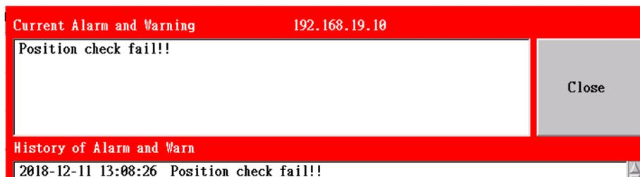
In order to conveniently use in the teaching procedure, the system pack the check as the additional G code. As long as the command of GM Code is used, G113 will be assigned and brought into the set order parameters A(0~3). If the check fails, the incorrect messages will be shown and the procedure execution will be stopped.
