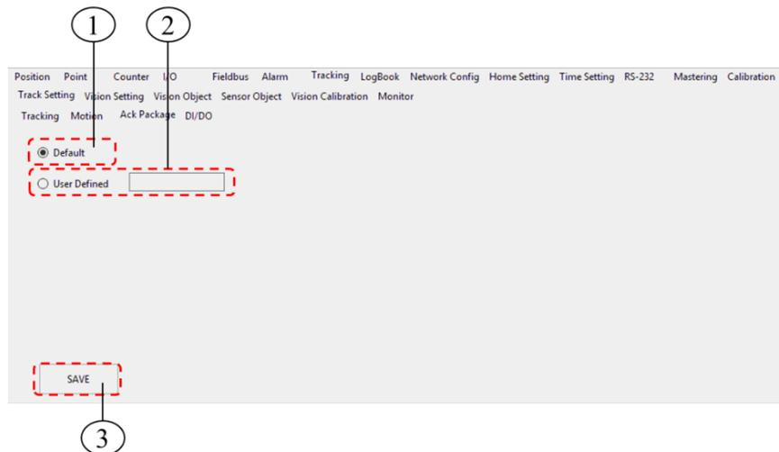
Conveyor Ack package parameters setting interface
