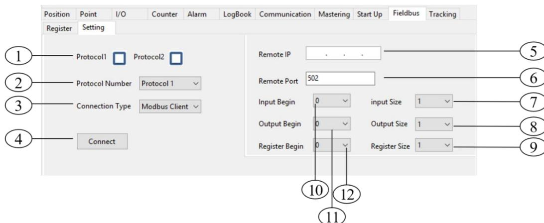
ModbusTCP Client connection parameters setting
