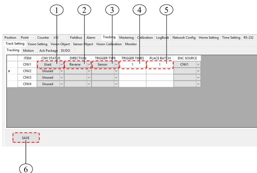
Conveyor tracking parameters setting interface
