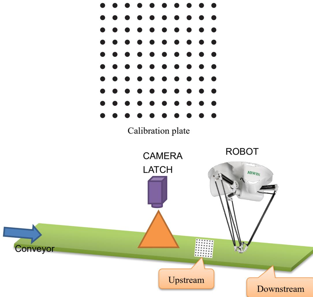
Illustration of Delta and CCD with conveyor
