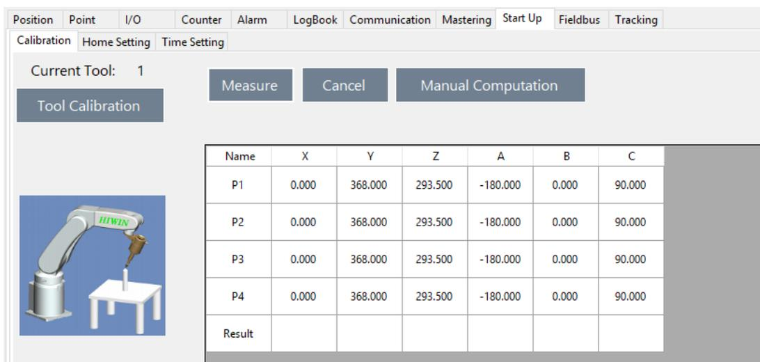
SCARA robot tool calibration interface
