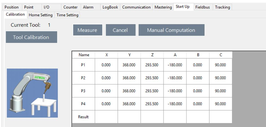
RA605 robot tool calibration interface
