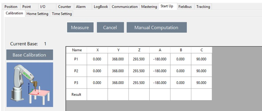
SCARA robot base calibration interface
