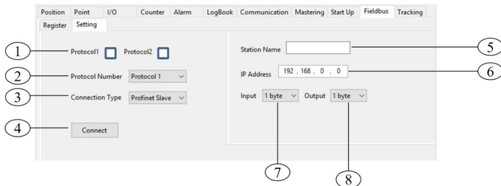
Profinet connection parameters setting
