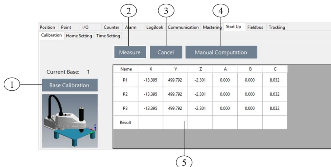
SCARA Robot Base/Tool calibration interface
