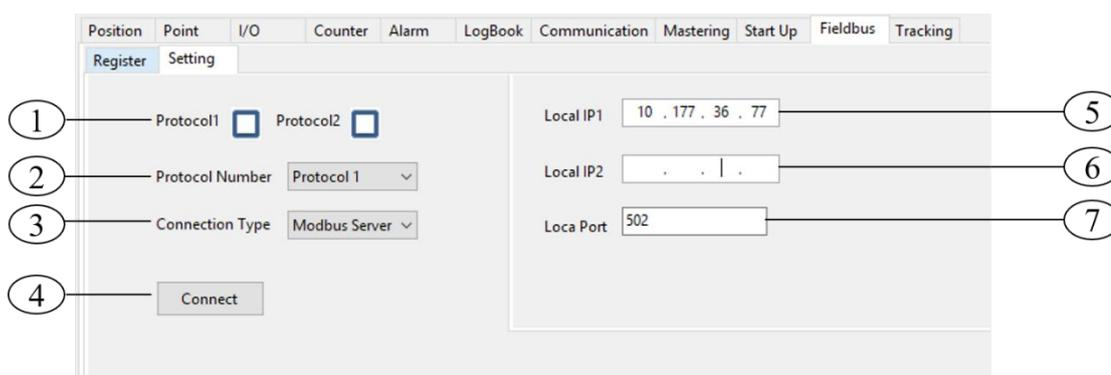
ModbusTCP Server connection parameters setting
