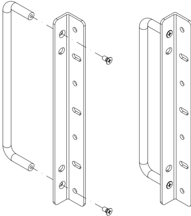
Multifunctional fixing frame can be installed on the controller. The assembly drawing is shown below. The specification of the screws is M6X1PX8L.
