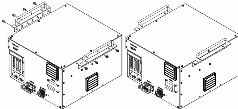
Multifunctional fixing frame can be installed under the controller. The assembly drawing is shown below. The specification of the screws is M6X1PX8L. This configuration is convenient for the operator to fix the controller on other machines.
