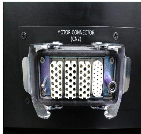
The motor power signal cable is connected to CN2 connector, and the safety lock is fastened.
